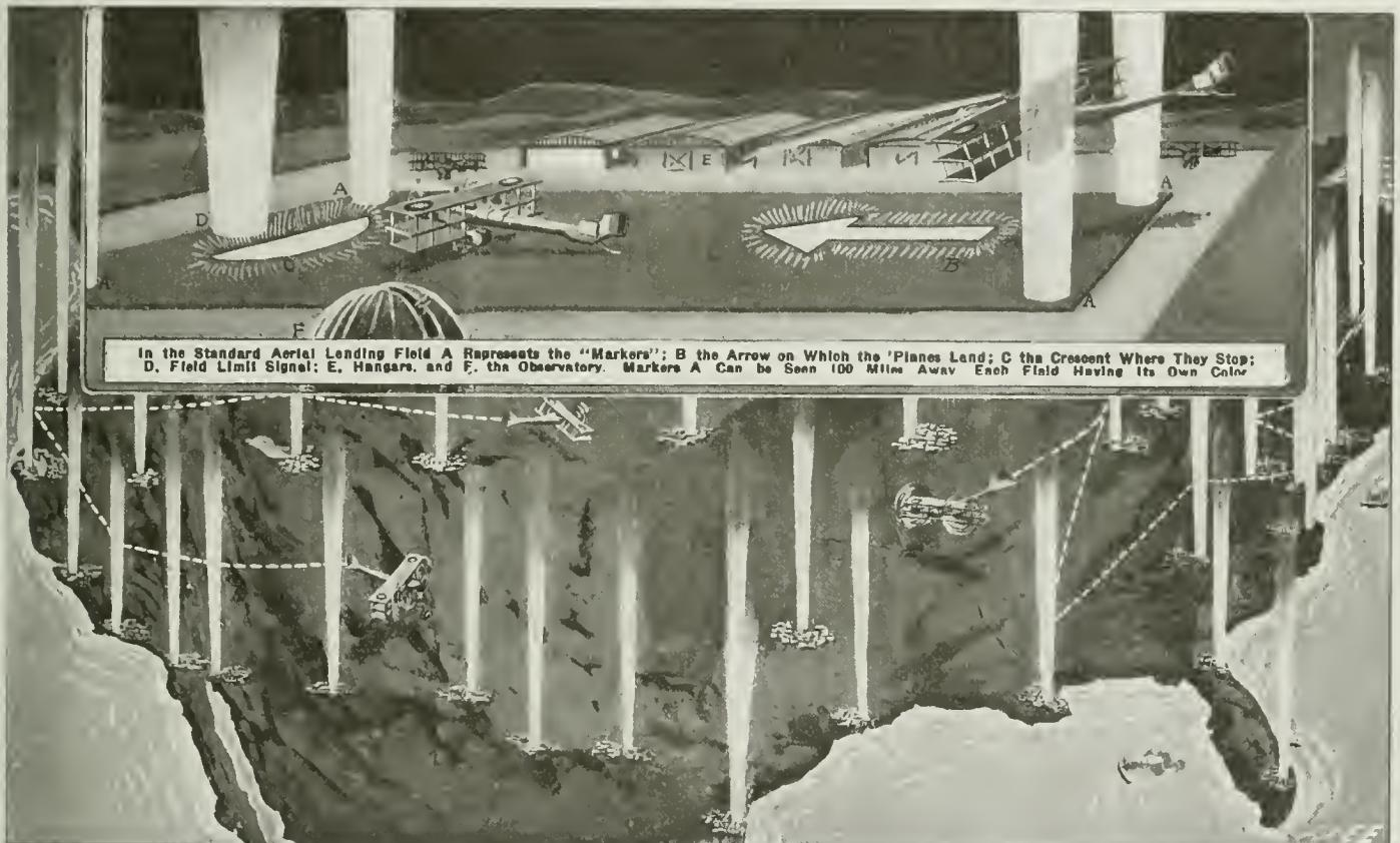
In the Standard Aerial Landing Field A Represents the "Markers"; B the Arrow on Which the 'Planes Land; C the Crescent Where They Stop; D, Field Limit Signal; E, Hangars, and F, the Observatory. Markers A Can be Seen 100 Miles Away Each Field Having Its Own Color
